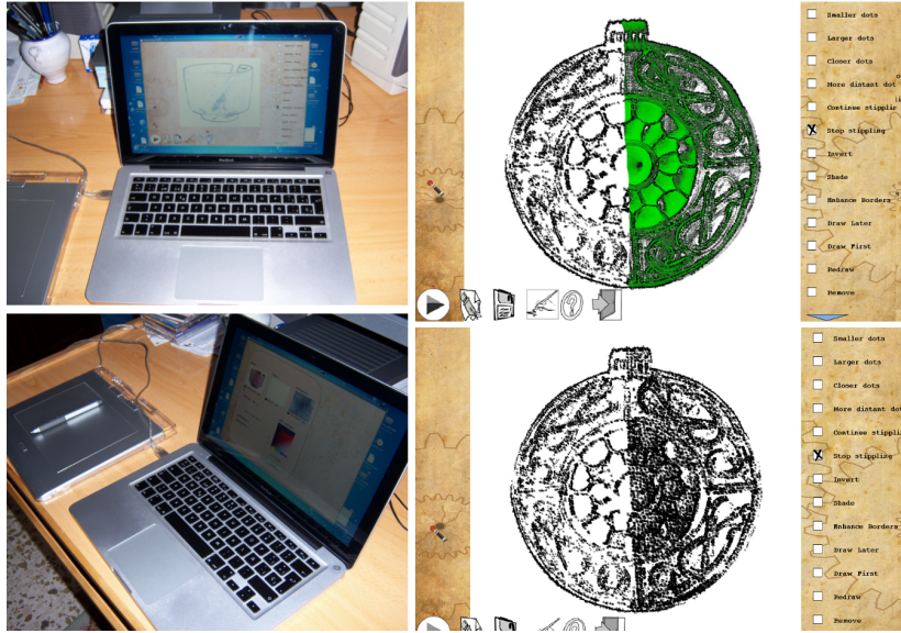
Figure 2: Our application executed in a laptop with a digital tablet (images on the left); the user can paint over a mask, which is presented in the image on the top-right corner. In this image, the mask indicates where to stipple and how to stipple, as shown in the bottom-right image.
