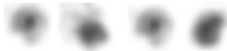
Fig. 2: From left to right, different scanned dots (600 dpi): A regular dot; an irregular dot; a mono-kernel dot; a multi-kernel dot.
