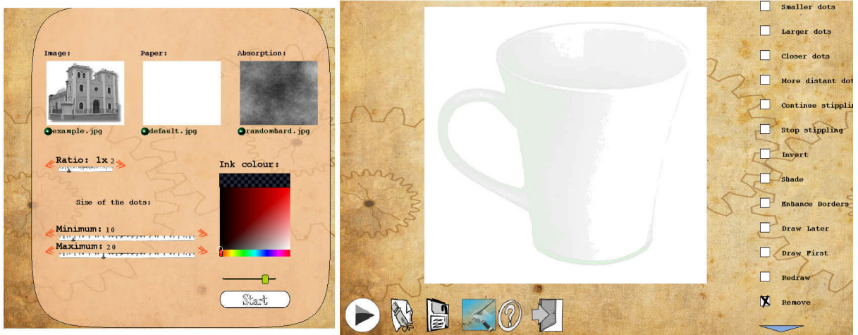
Fig. 8: (Left) a screenshot of the main interface; it allows the user to select the size and color of the dots, the input photograph, and the absorption of the paper. (Right) a screenshot of the interface for automatic stippling; it shows the mask of the photograph as a background for placing the dots when the algorithm continues. The options on the right menu show the different tools for editing the stippling process (from top to bottom): Smaller dots, Larger dots, Closer dots, More distant dots, Continue stippling, Stop stippling, Invert, Shade, Enhance borders, Draw later, Draw first, Redraw, Remove.
