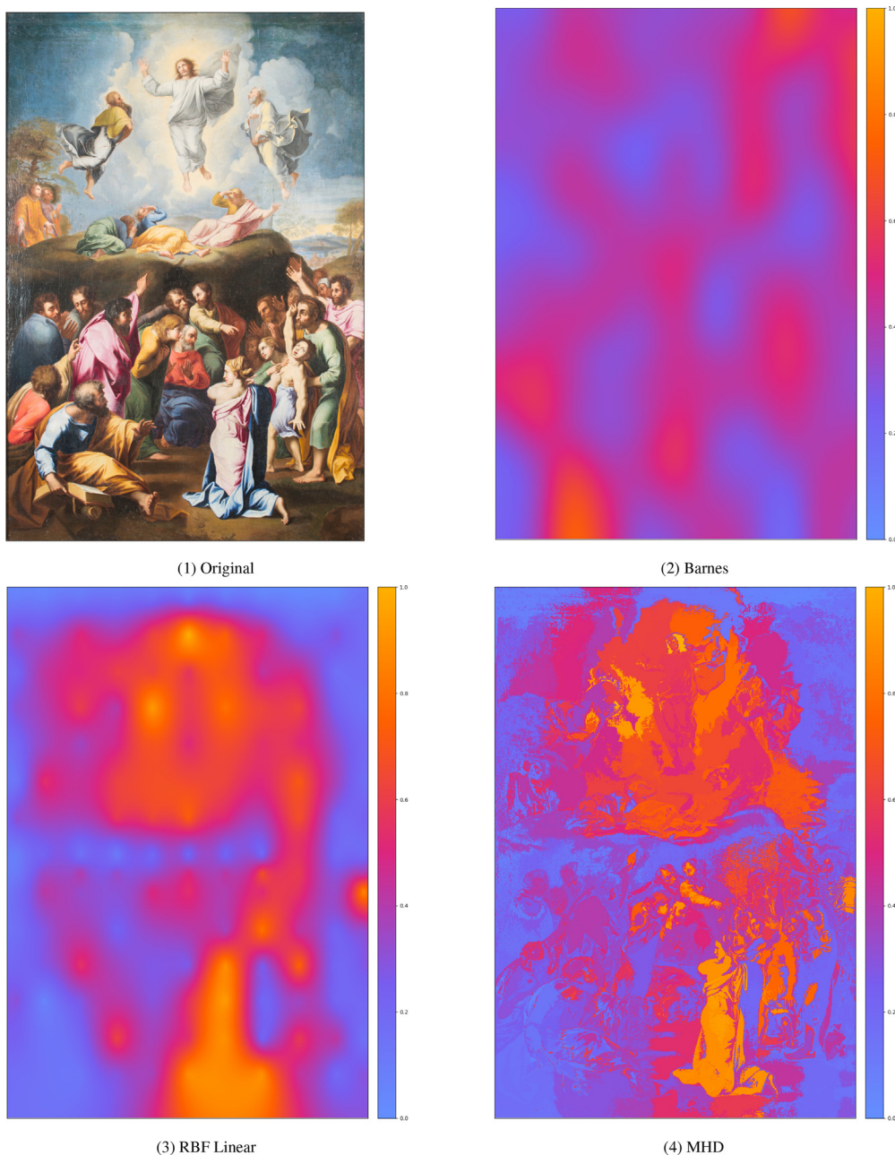
Fig. 8. Example of interpolation maps for Pb element using an input image of 756 pixels × 1112 pixels (W × H) and all the measured values, 165, of “The Transfiguration” dataset.
